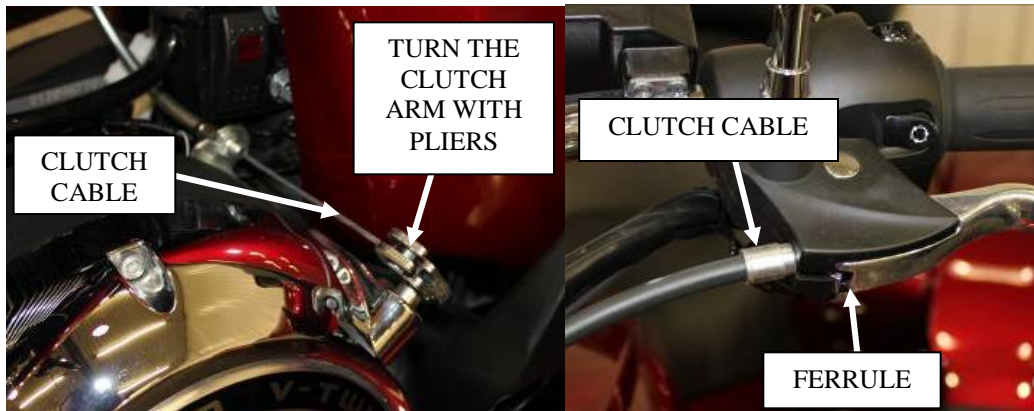
Figure 11: Remove the clutch cable from the clutch arm and the handlebar.
