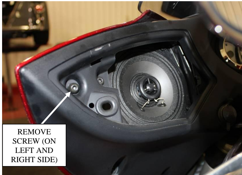
Figure 6: Remove the screw under the speaker grill.
