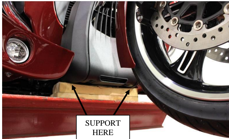
Figure 1: Support the front of the motorcycle and lift the front tire.
