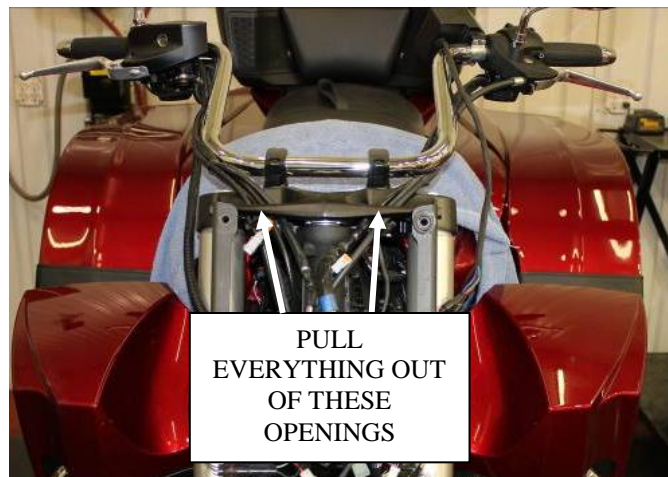
Figure 10: Remove the brake line, wiring, and clutch cable from the openings on the front of the triple tree.
