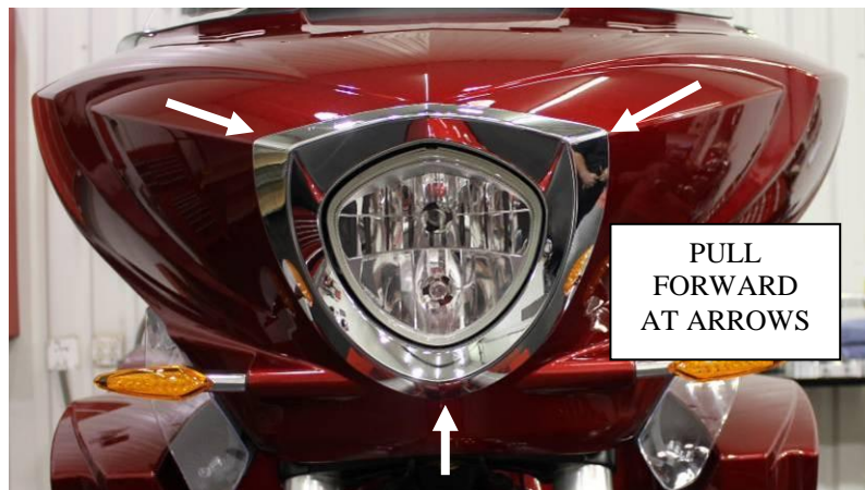
Figure 2: Pull the bezel off the front headlight.
