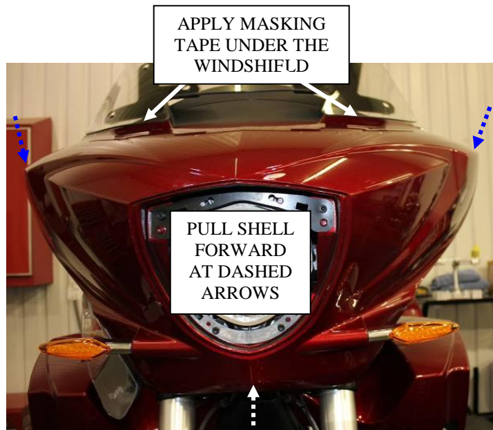
Figure 7: Remove the outer shell of the fairing.
