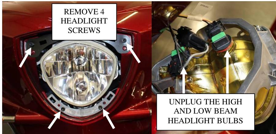
Figure 3: Remove the headlight and unplug the connectors.
