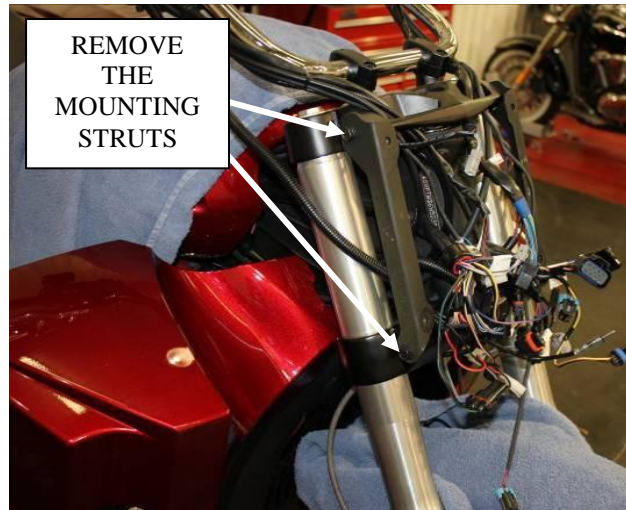
Figure 9: Remove the fairing mounting strut from the triple tree assembly.
