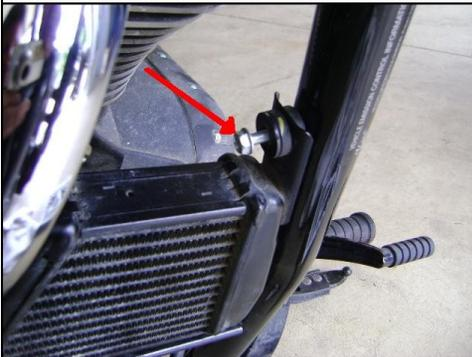
1) Remove the 10mm bolt that secures the oil cooler to the frame.
