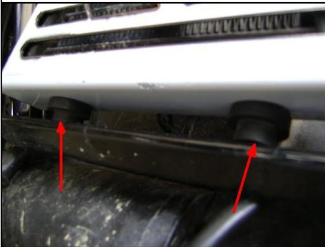
2) Gently lift up on the oil cooler. Make sure the rubber vibration mounts stay in the crossbar. Slide the bottom of the cooler cover between the cooler and rubber mount.
