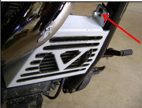
3) Slide the top of the cooler in place. Reinstall the 10 mm bolt through the cooler cover and tighten. Check for clearance and fitment on exhaust. After a few miles of riding check for movement and to make sure bolt is tight.
