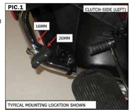
STEP 6 Ensure that the position of the Toe Rest does not interfere with the proper operation of the motorcycle BEFORE riding.
